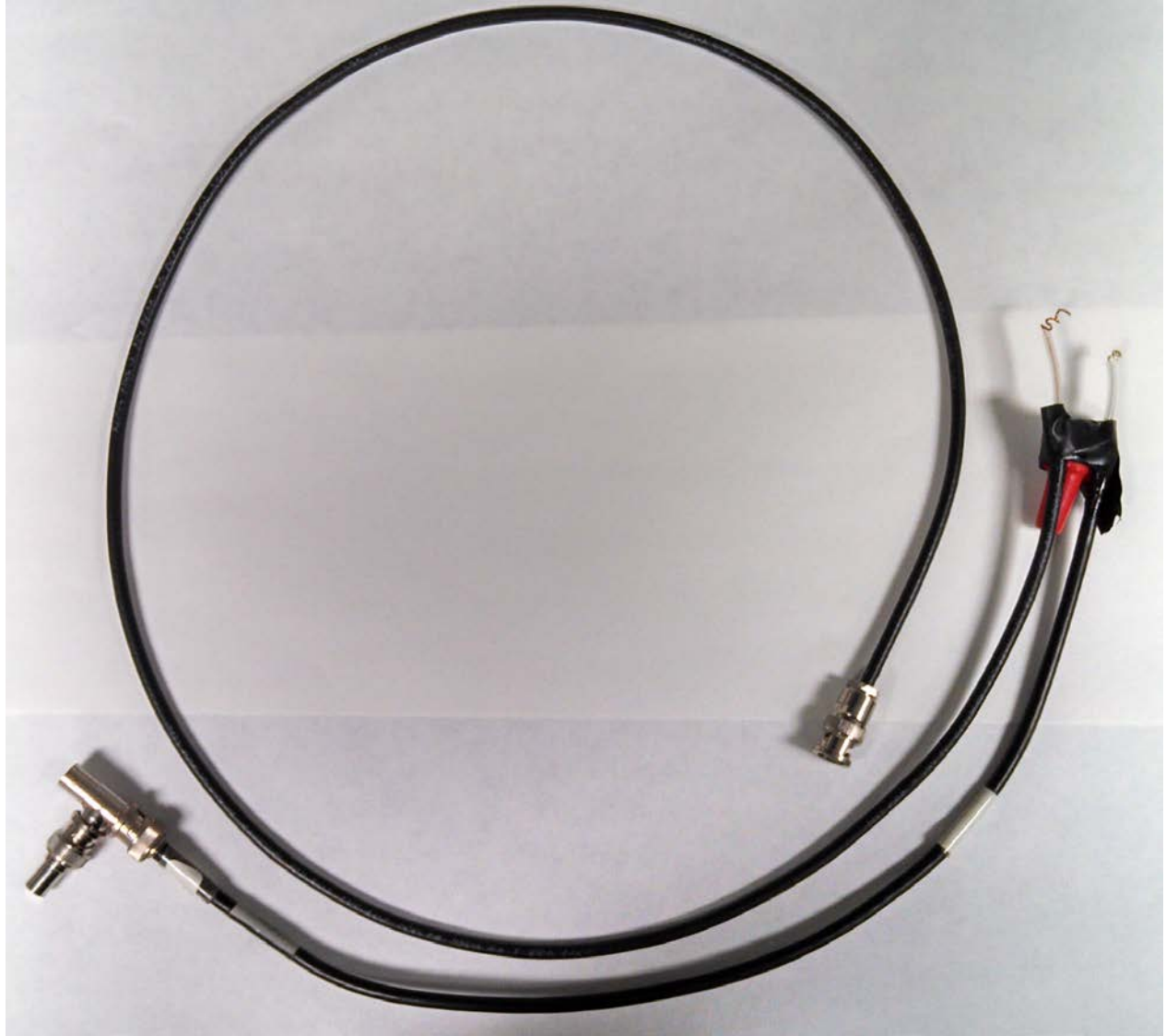
Figure 4.6 The spliced coaxial BNC cable for measuring the current flow to the scanning etalon. At the open end on the right, the cladding has been joined together in the red wire tie and wrapped in electrical tape. The center core is left bare to connect to the multimeter and read out the current.
